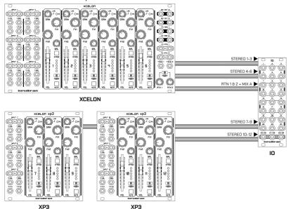
This configuration provides eurorack-level direct outputs for the entire Xcelon mixer system. Signals can then be selectively patched from IO into an audio interface or to other destinations.
